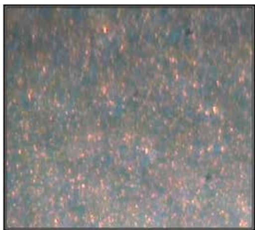
Figure 3: shows the effects of the radon-free alpha particles in the impact detector (CR-39)
